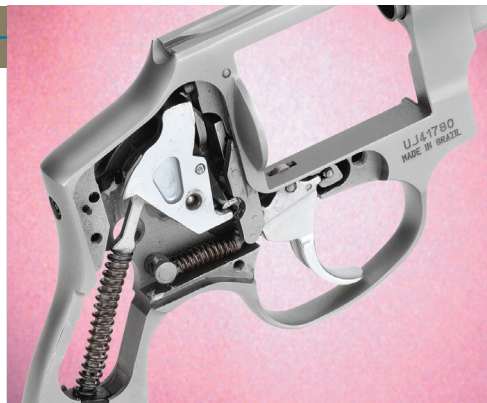
The feature that really sets the CIA apart from Taurus' previous offerings is the fact that it has an internal concealed hammer much like the S&W Centennial revolvers. The rear sight (above r.) is merely a fixed notch in the top rear of the frame.
