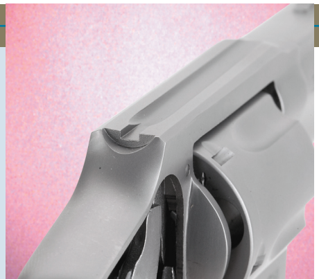
The feature that really sets the CIA apart from Taurus' previous offerings is the fact that it has an internal concealed hammer much like the S&W Centennial revolvers. The rear sight (above r.) is merely a fixed notch in the top rear of the frame.
